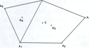
$$\begin{aligned} \text{Area } A_1A_4A_5 &= 10.315 \text{ cm}^2 & CG_4 \cdot (\text{Area } A_1A_4A_5) &= 27.095 \text{ cm}^3 \\ CG_4 &= 2.627 \text{ cm} & CG_3 \cdot (\text{Area } A_1A_2A_3A_4) &= 27.095 \text{ cm}^3 \\ \text{Area } A_1A_2A_3A_4 &= 24.434 \text{ cm}^2 & CG_3 &= 1.109 \text{ cm} \end{aligned}$$
