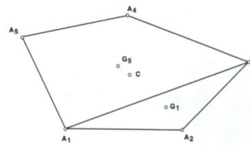
$$\begin{aligned} \text{Area } A_1A_2A_3 &= 7.958 \text{ cm}^2 & CG_1 \cdot (\text{Area } A_1A_2A_3) &= 17.088 \text{ cm}^3 \\ CG_1 &= 2.147 \text{ cm} & CG_5 \cdot (\text{Area } A_3A_4A_5A_1) &= 17.088 \text{ cm}^3 \\ \text{Area } A_3A_4A_5A_1 &= 26.791 \text{ cm}^2 & CG_5 &= 0.638 \text{ cm} \\ CG_5 &= 0.638 \text{ cm} \end{aligned}$$
