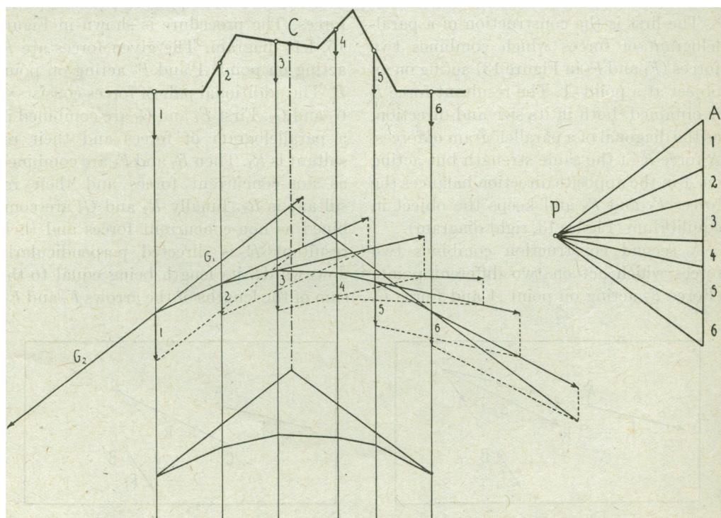
FIG. 16. Derivation of the construction of the centroid by force and equilibrium polygons.
