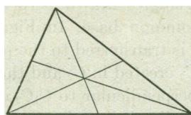
FIG. 1. Centroid of a triangle.
