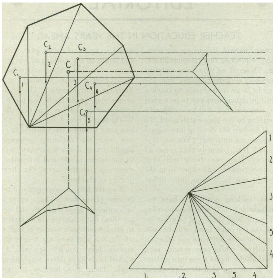
FIG. 17. Construction of the centroid of an area through force and equilibrium polygons.
