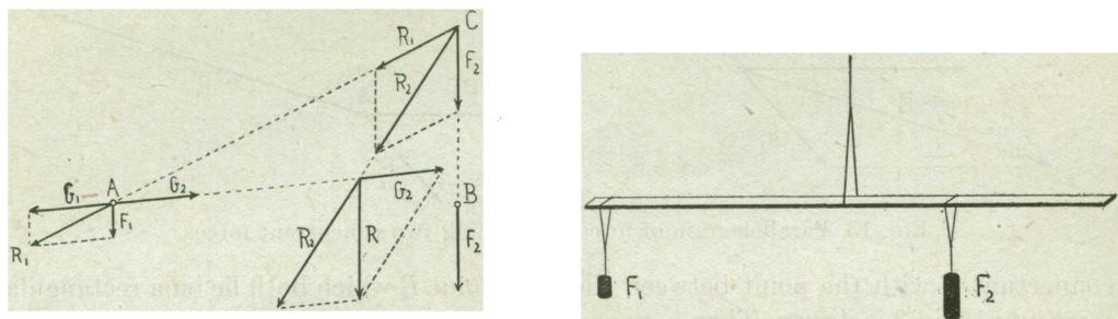
FIG. 15. Resultant of two parallel forces.
