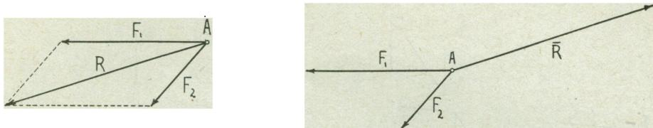
FIG. 13. Parallelogram of forces combining two concurrent forces.
