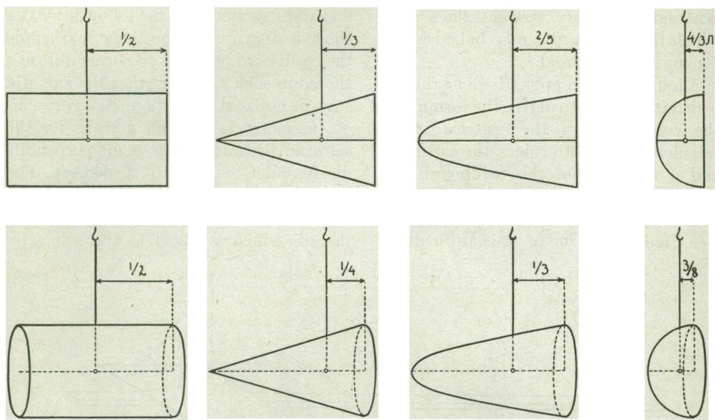
FIG. 11. Suspending of areas and solids in horizontal position.
