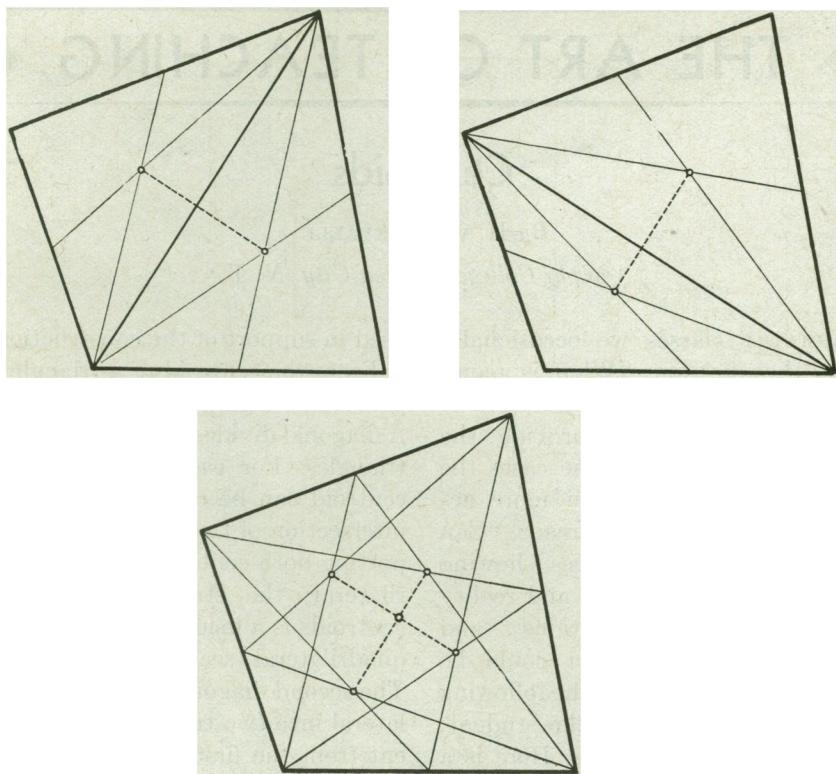
FIG. 2. Centroid of a quadrilateral.
