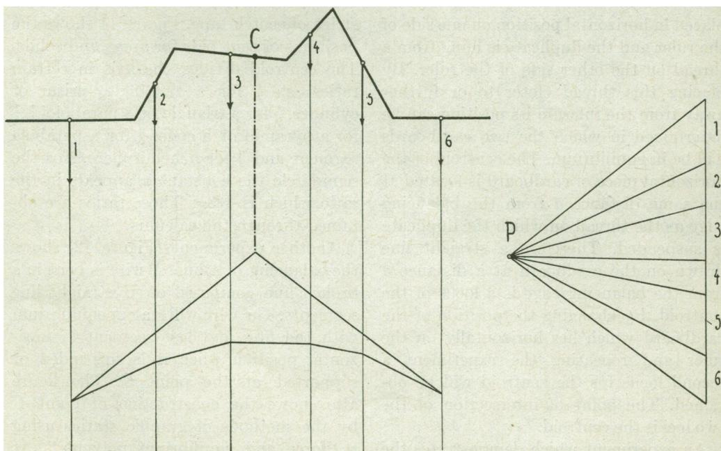
FIG. 12. Balancing of a broken line.
