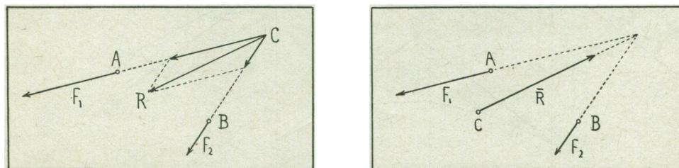
FIG. 14. Parallelogram of forces for two non-concurrent forces.
