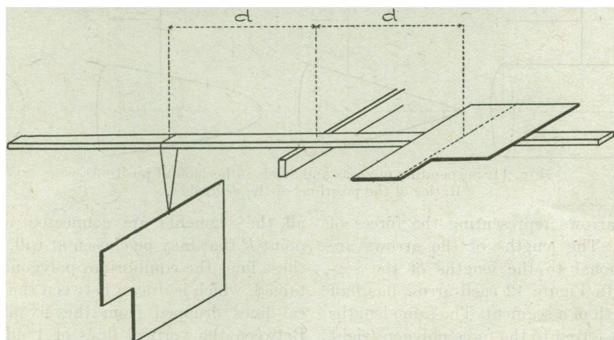
FIG. 10. Experiment to find the centroid of a cardboard-area.
